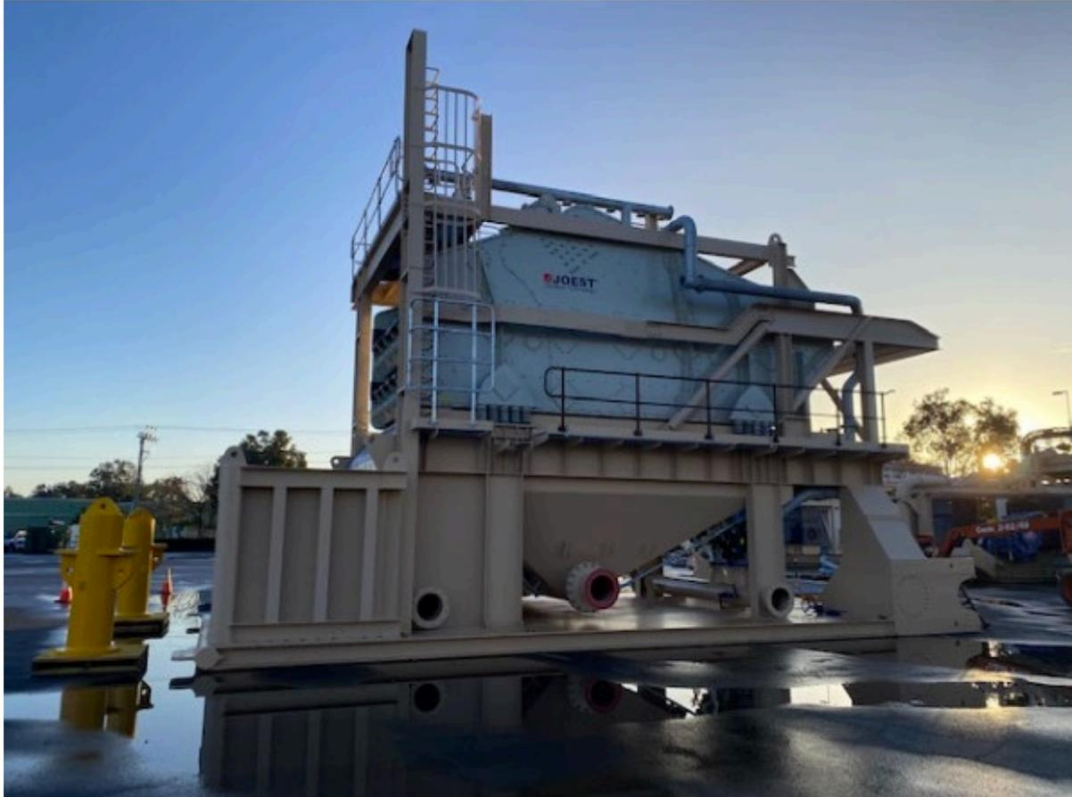
Image 5: Dry Mining Unit Screen Assembly
