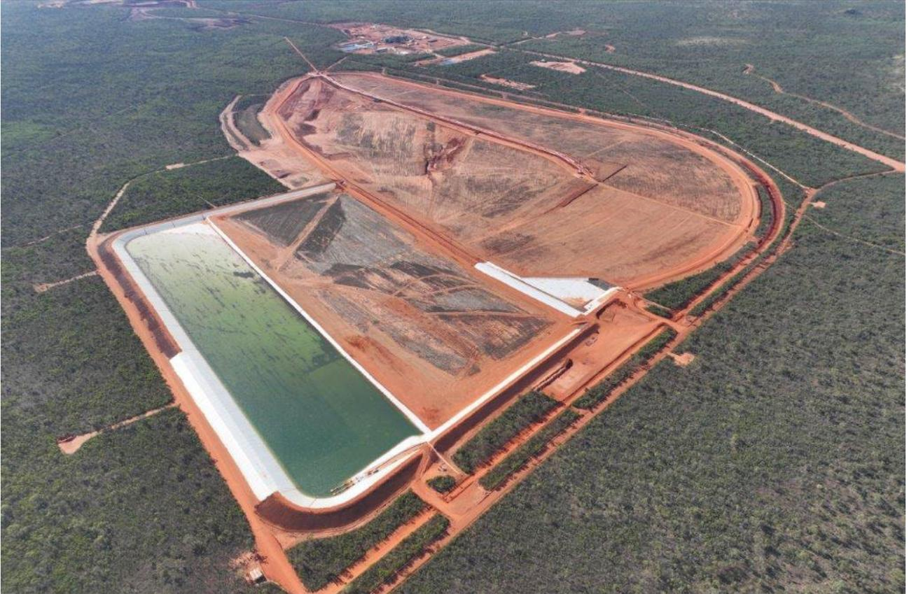
Image 3: Tailings storage facility & stormwater storage pond (foreground)
