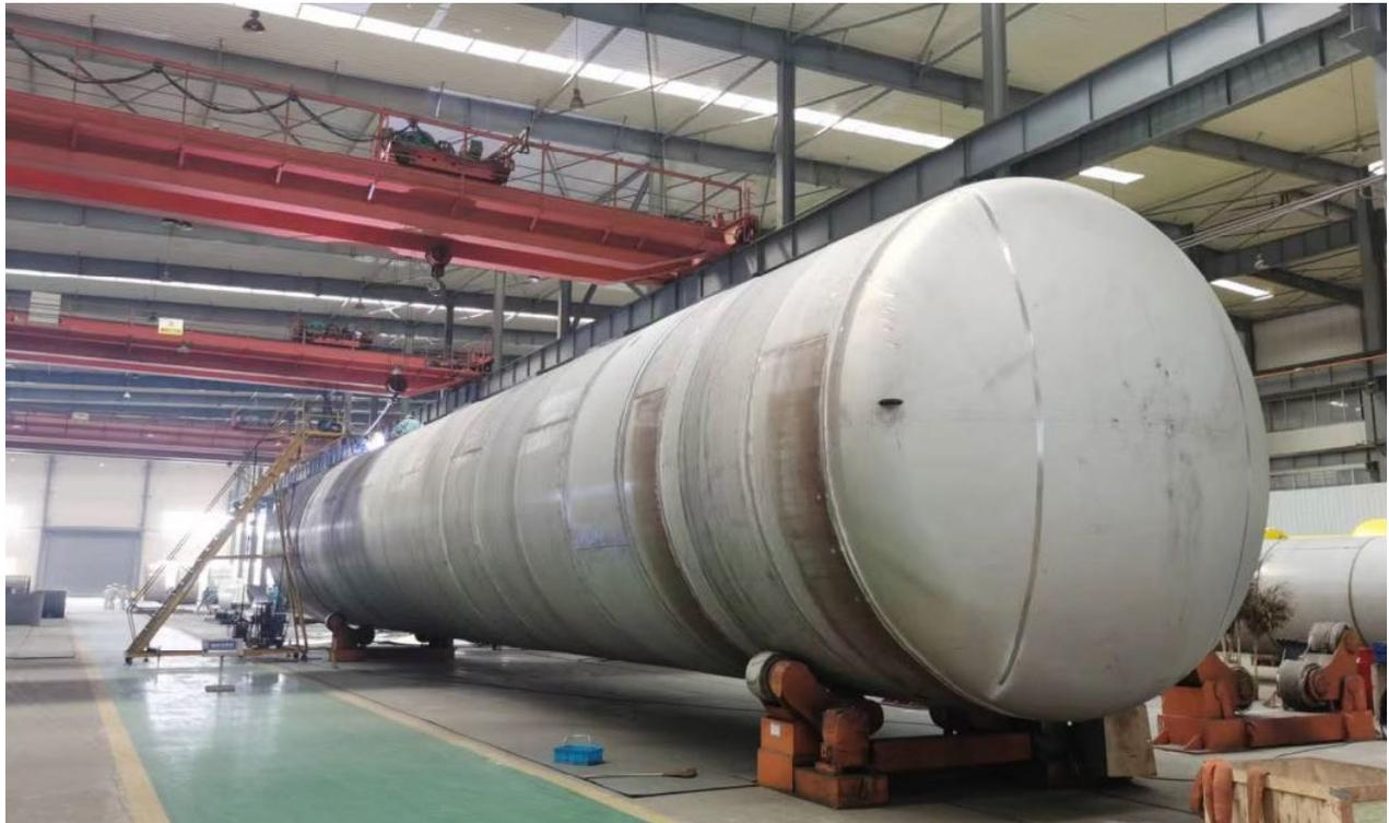
Image 2: Thunderbird Project - LNG storage tank fabrication
