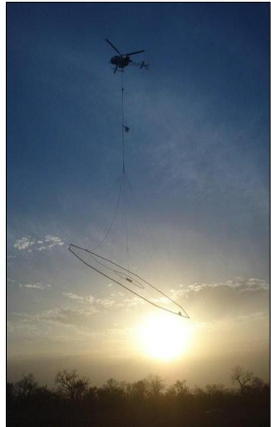
**Figure 3: Example of Geotech's VTEM system in action (photo courtesy of Geotech Airborne Pty Ltd).**
